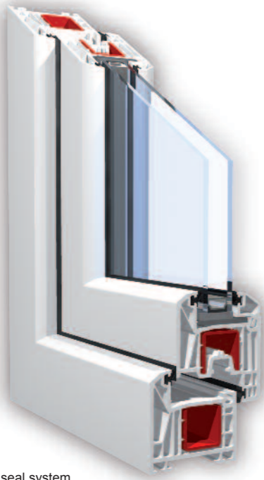
Five chamber double seal system with 70 mm installation depth
